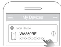
4. Follow app instructions to complete the setup. The RE LED should turn solid on, indicating successful connection to your router.
