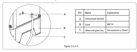
4. In order to improve the corrosion resistance of the terminal, it is recommended to apply silica gel on the earth terminal for the corrosion protection after the grounding cable assembly is completed.
