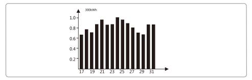
300kWh means the maximum power generation of recent 16 days. The unit on the left corner sometimes turns to "MWh" from "kWh", it depends on Maximum power generation. 0.2~1.0 on the left is scare factor, which is fixed display content; 17~31 are based on current mode which shows the bar chart label.
