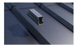
**Caution!** Install the steel roof bracket on a high part of the steel roof. The water drainage passes through the lower part.
